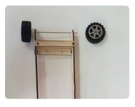
5) Put an axle in a wheel. Slide the axle through the axle hole in side A, on the same end of the racer as the C connector, then through the axle hole in side B. Add a wheel on the other side of the axle.
