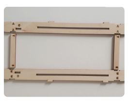
2) Place 2 sides and 2 AB braces on a table with the letters facing up. Insert the braces into the bottom notches on side A, matching the letters on the braces with the letters on the bottom notches. Glue in place.
