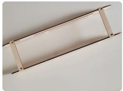
3) Repeat with side B. Repeat with the upper braces - attaching the letters on the braces with the letters on the sides. Remember to hold the pieces together for 30 seconds when gluing.
